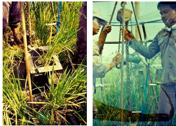
Fig. 8. IRRI monolith sampler setup (left; IRRI 1985). Monolith samplers were used in well-watered treatments and lifted from the soil profile using a suspended chain block (right; photos from Ofelia Namuco).
