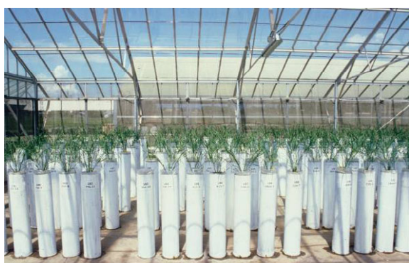
Fig. 9. Large (about 1 m tall) PVC cylinders were used in greenhouse root studies starting in the 1990s. Photo from Brigitte Courtois.
